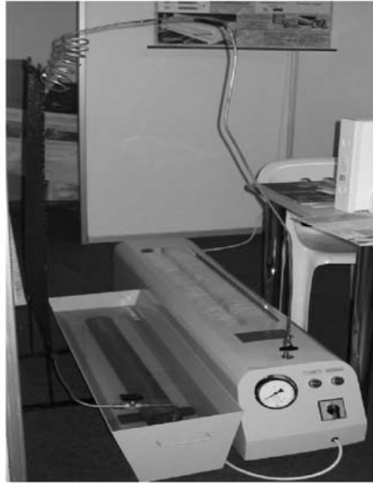
Fig. 4. Sorption heat pump for heating of air and cooling of water of power 4 kW (heat) and 1 kW (cold), designed at the Heat and Mass Transfer Institute of the National Academy of Sciences of Belarus.
